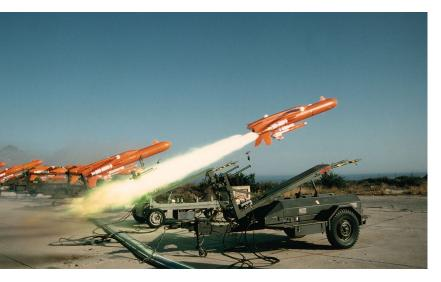
The updated Mirach 100/5 is an evolution of the successful Mirach 100/5 featuring a range of mid-life upgrades, including PBS TJ150S engine, advanced new avionics and enhanced re-liability.
