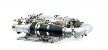
ECS FOR SMALL TURBOPROP AIRCRAFT
